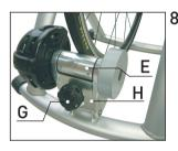
8. Before proceeding make sure that the rear tire of the bike is properly inflated. Check the sidewall of the tire for the manufacturer's recommended pressure range, and inflate accordingly. Using the Adjustment Knob **"G"** set the Magnetic Resistance Unit **"H"** so that the roller contacts the bike's rear tire. Then turn the Adjustment Knob **"G"** clockwise two full turns to insure that you have sufficient pressure of the Drive Roller "E" on the rear tire.
