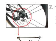
2. Replace the quick-release skewer on the rear wheel of your bike with the Quick-Release Skewer "M" included with the trainer. This assures ideal clamp fitting and stability.
