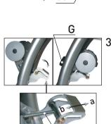
**3.** The Linkage Pillar **"J"** is controlled by the Wheel Adjustment Knob "G". Try to move linkage pillar from frame attachment stay tracking location (a) to (b) until it's locked.
