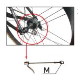
**2.** Replace the quick-release skewer on the rear wheel of your bike with the Quick-Release Skewer "M" included with the trainer. This assures ideal clamp fitting and stability.
